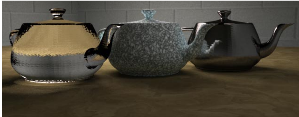
Figure 4.2: Three teapots illustrating different Shader types. From left to right are a perfectly specular transparent shader, a diffuse shader using a 3D Perlin noise texture to simulate marble, and a phong shader with an exponent of 2048. Rendered with a path tracer using 400 samples per pixel. Note the very soft shadows, indirect illumination and caustic cast by the leftmost teapot.
